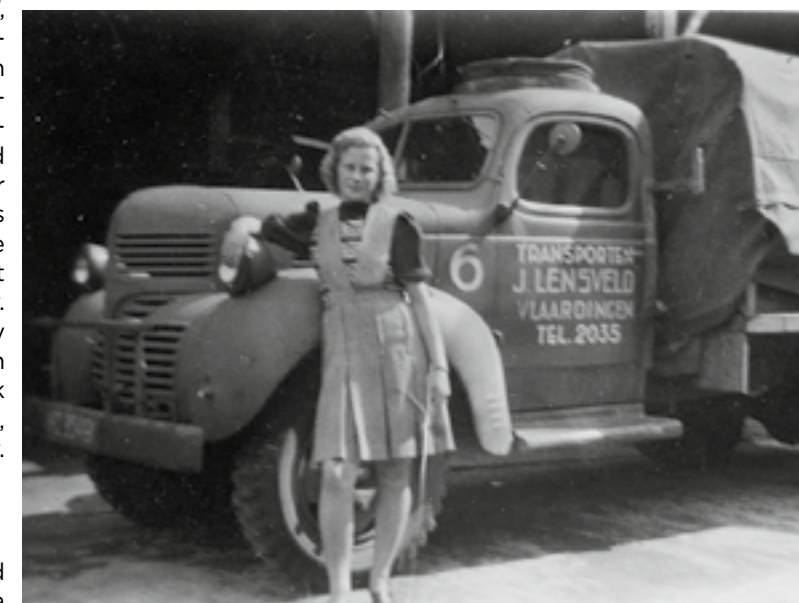
Jan's daughter Maartje in front of a Canadian Dodge T110. The gunner's hatch is still visible atop the cabin.
