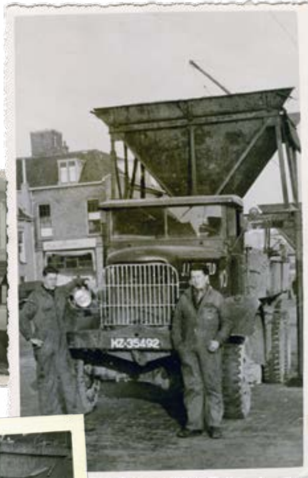
Mari and Van Leeningen in front of a MACK NM 6-tonne truck.
