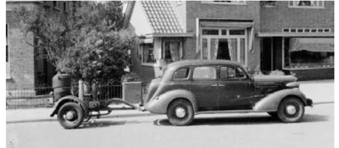
Car with gas generator. Photo: The Niestadt bros. Memory of the Netherlands collection.
